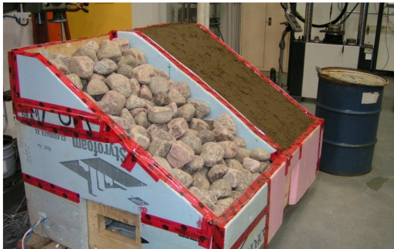
Figure 2.2 Embankment box with the two small-scale embankments, air convection embankment and reference embankment
