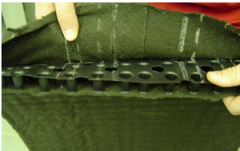
Figure 2.16 The geocomposite, which is used to extract heat out of the embankment (Beaulac and Doré, 2006-B)
