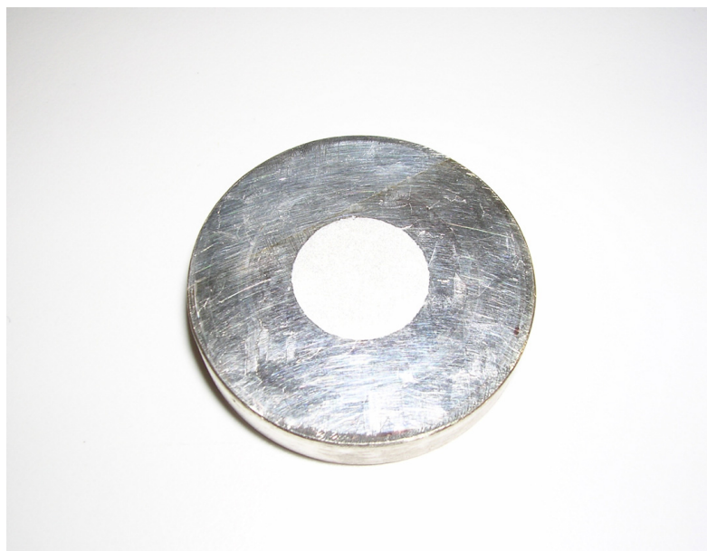
Figure 3.2: Electroplated tin target (Ø10mm) on a silver backing (Ø29mm, 5.2mm thickness)
