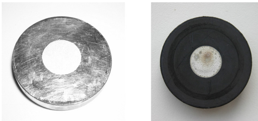
Figure 4.3: Electroplated tin targets on silver and graphite backings using the alkaline plating solution. The tin target with the graphite backing had been irradiated with 16 MeV protons before this picture was taken. Hence, the brown spot on the tin.
