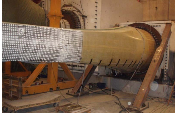
Figure 4. Box girder 2 mounted in test rig. Note there is no tophat reinforcement as in the first box girder test, see reference [2]
