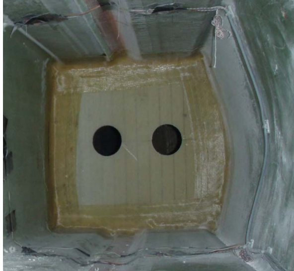
Figure 8. Rib in 13.20m manufactured and bounded by SSP Technology A/S.
