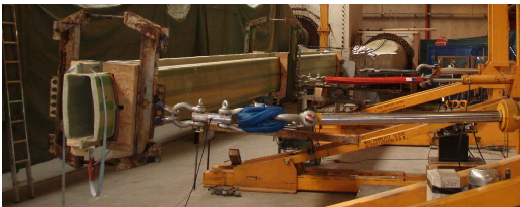
Figure 3. Box girder no 2 ready to be tested in flapwise bending. The box girder was shortened to 25.4m.
