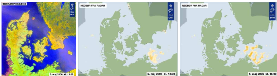
Figure 1.2: Clutter is a common unwanted feature of weather radar data. The satellite image on the left (from a NOAA polar-orbiting weather satellite) shows cloud-free conditions, while the two radar images (middle and right), as presented on the DMI website, show radar clutter (patches in yellow hues) in the Baltic Sea.
