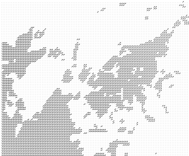
Figure 4.5: HIRLAM wind field. The direction of flow is homogeneous for the whole region. The speeds were normalized to 1 for clarity.
