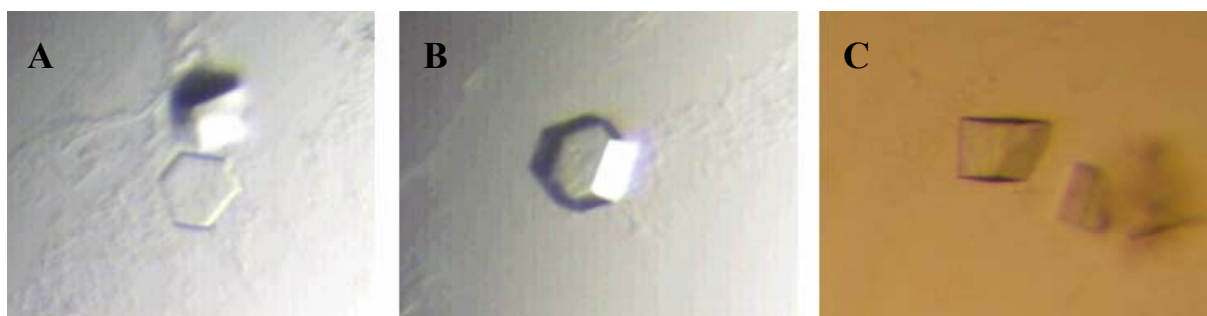
Figure 3.3 Crystals of dCTP deaminase dUTPase crystallized in the presence of \alpha,\beta -imido dUTP. All crystals are from plate C2 number A5 (appendix A.3). The crystals are ca 40 \mu\text{m} on the longest axis. The crystal shown in B was used for data collection.
