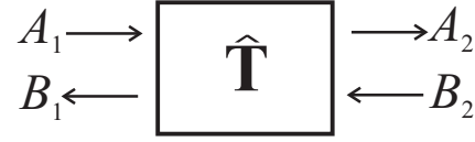
Fig. 2.7: Definition of the transmission matrix \hat{\mathbf{T}} . The matrix relates the forward ( A_j ) and backward ( B_j ) traveling waves.
