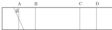
FIG. 11. Top-view schematic of chip and blades (A)–(D). In the FEM analysis, each blade is rotated an angle \phi . The stress distribution for different configurations of blade rotation is listed in Table II.
