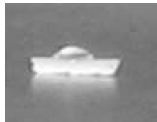
Figure 8: 10 \mu\text{l} droplets of water on a PES/PVP hollow fiber surface.
