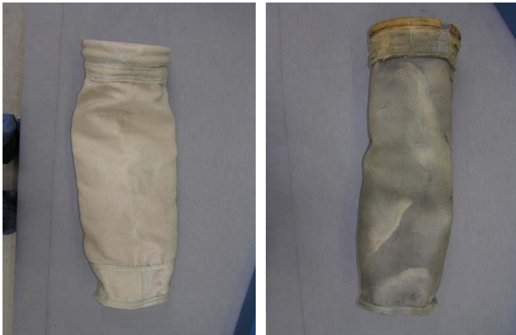
Figure 4.18 Picture of an unused bag and a bag after the filtration experiments
