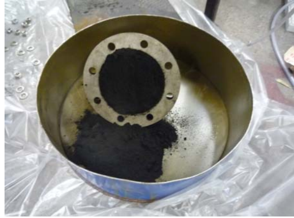
Figure 4.15 Ash & sand particles collected from the bottom of the gas cooler
