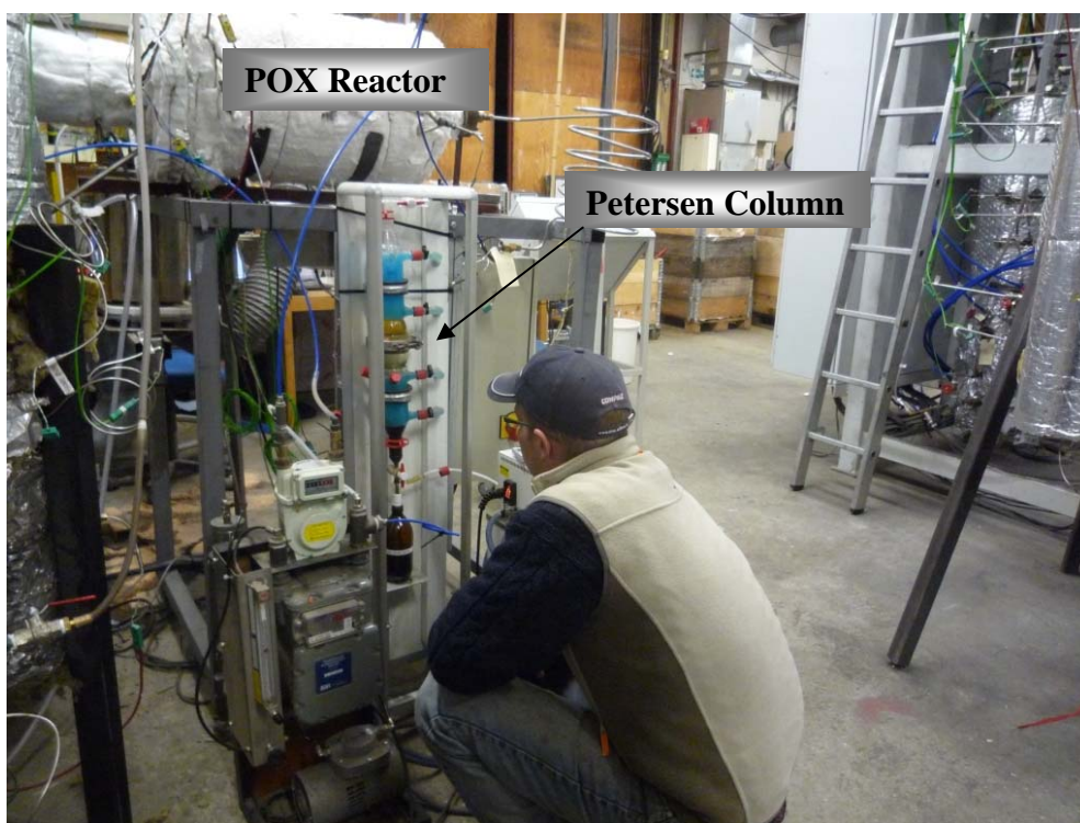
Figure 4.10 Partial oxidation (POX) and tar sampling setup
