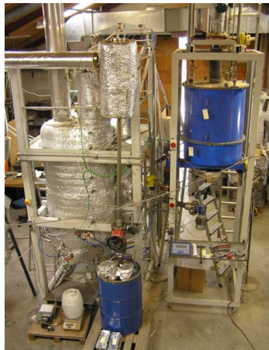
Figure 2.14 100 kW th LT-CFB gasifier
