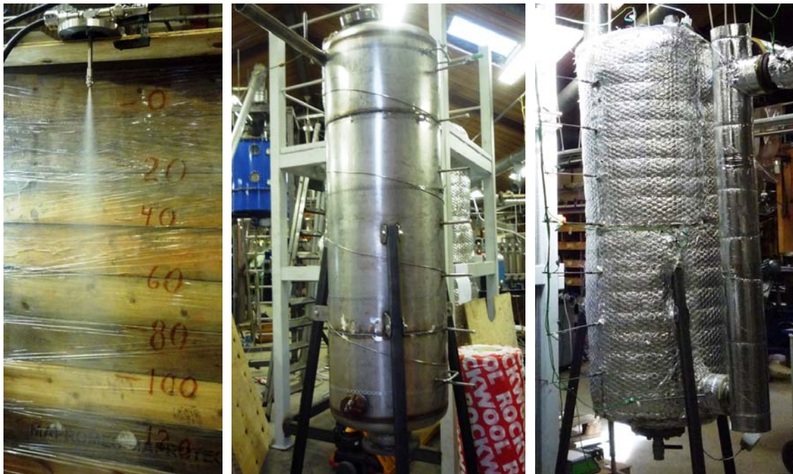
Figure 4.4 Test of nozzle (left), evaporative cooler without insulation (centre) and evaporative cooler with insulation (right)
