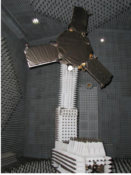
Figure 1. Central part of the MIRAS, consisting of the hub and the three inner arm segments, on the tower of the DTU-ESA Spherical Near-Field Antenna Test Facility during the last measurement series.
