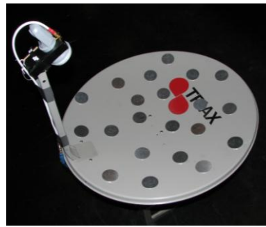
Figure 14. Offset reflector with surface distortions.
