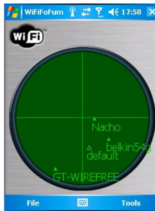
Figure 6-19: Screen shot of WLAN access point location detection using WiFiFoFum ( Aspecto Software 2007 ).
