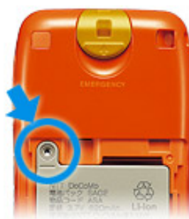
Figure 5-2: Battery lock of the child friendly terminal designed for imadoco search service (NTT DoCoMo 2007b).
