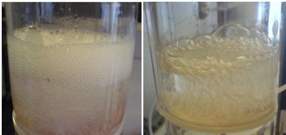
Figure 5.2: Foaming behaviour illustrated by 10 -2 M adipic acid solution (left) and the bubble transition layer formed in the absence of foaming illustrated by demineralised water (right). Both have a velocity of u_{su} = 0.01 \text{ m s}^{-1} .
