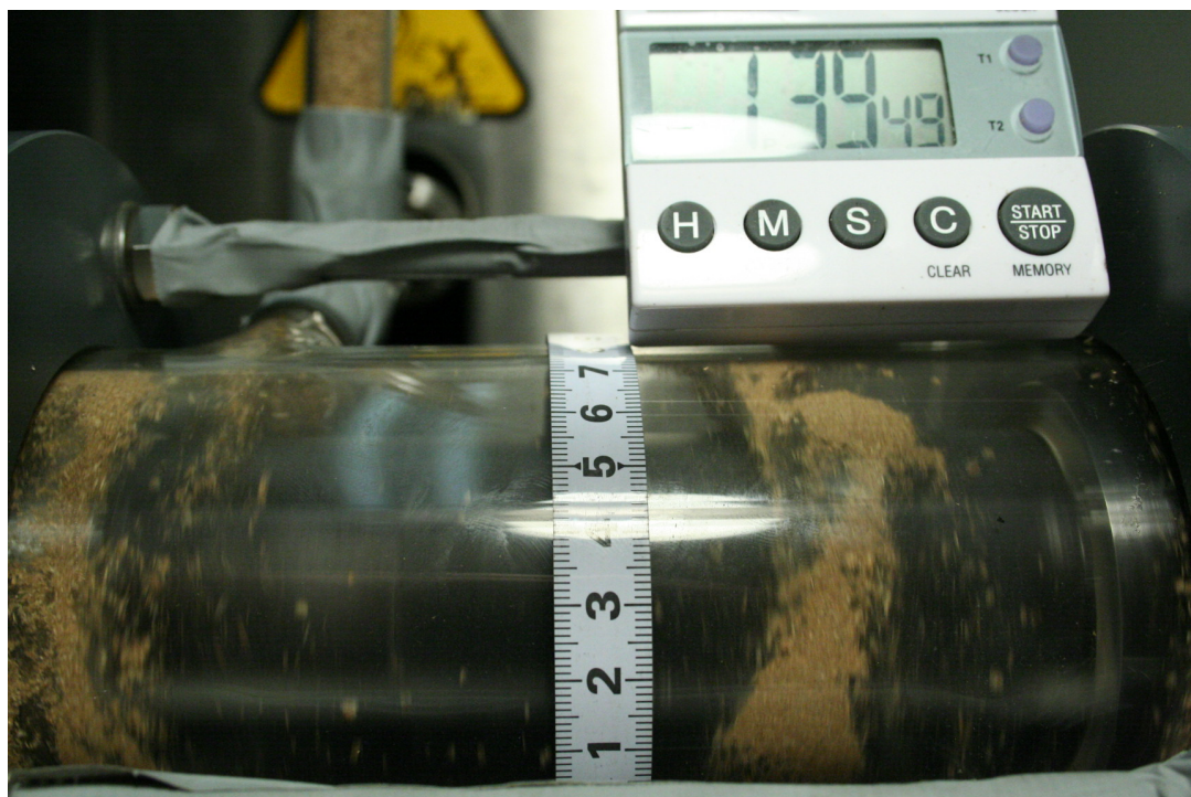
Figure 2: Picture of the material flow in the unmodified glass reactor taken with an exposure time of 1/4000 s, feed rate 23 \text{ g s}^{-1} , and rotor speed of 14,784 rpm. The feed port is to the left and a “ring” of material (below the timer) has just separated and is rapidly moving towards the outlet in the lower right corner (out of view). In this picture the rotor has been fitted with end rings that limit the accumulation of material to the left of the feed port.
