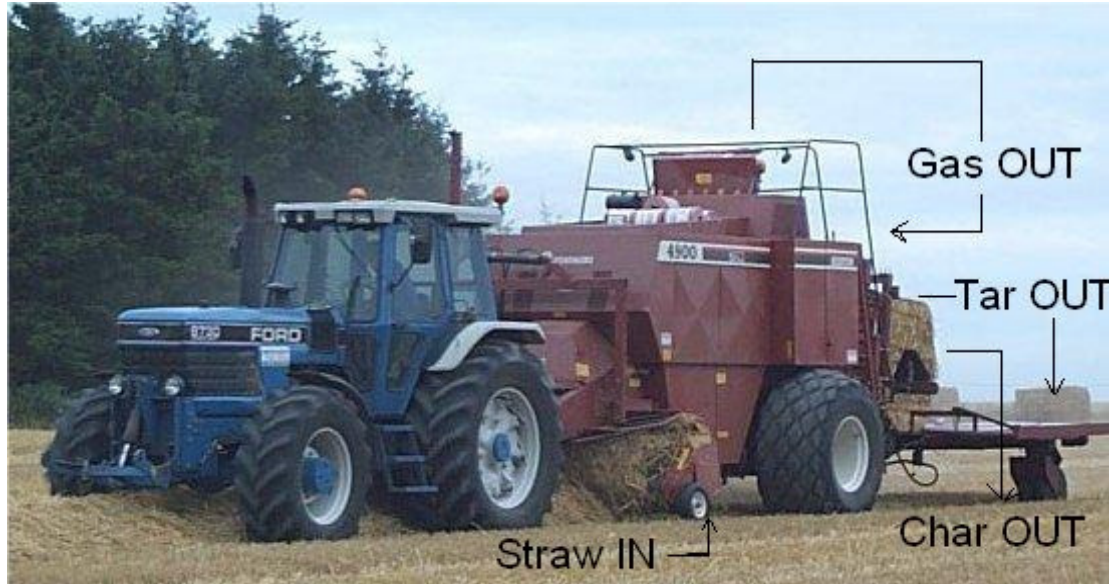
Figure 2: Schematic presentation of the pyrolyzer in operation on the field. Straw is processed by flash pyrolysis in the pyrolyzer pulled by the tractor to obtain gas, tar (bio-oil), and char. The gas is combusted internally to provide process heat, whereas char is distributed on the field. Bio-oil is collected on board and transferred to a transport vessel on the field when full [3, 4].
