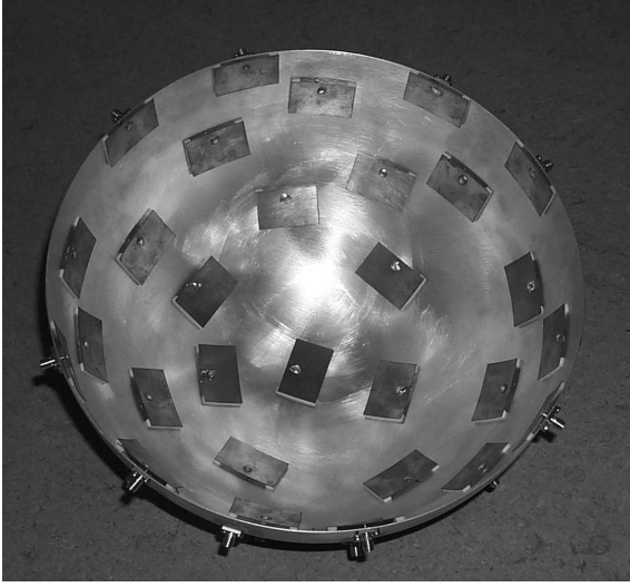
Figure 1. Picture of the PAT scanner. The system is designed to work at the frequency 5 GHz and consists of a aluminum hemisphere inside of which is positioned conformal patch antennas made of copper plating.
