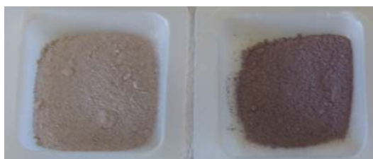
Figure 7.1.: Two gold catalysts, 1 wt% Au/ \text{MgAl}_2\text{O}_4 , 1.5 wt% Au/ \text{TiO}_2
