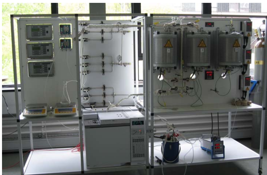
Figure 4.2.: Example of an experimental setup for steam reforming of ethanol, here with three parallel reactors.
