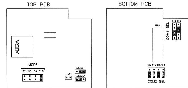
In the jumper configuration tables below the jumper text labels can be used to indicate the orientation of the jumpers.
