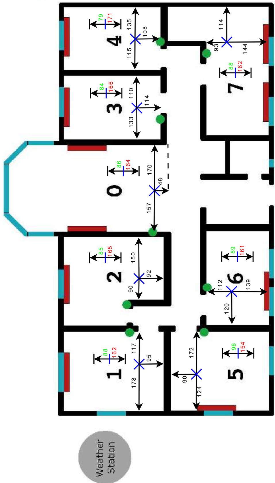
Figure B.2: The position of the Hobos. All lengths are in centimeters. The red numbers indicate the height from the floor to the sensor, and the green number indicate the height from the sensor to the ceiling.
