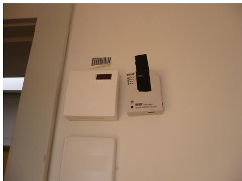
Figure 5.7: A Hobo hanging next to a the wall mounted temperature sensor.
