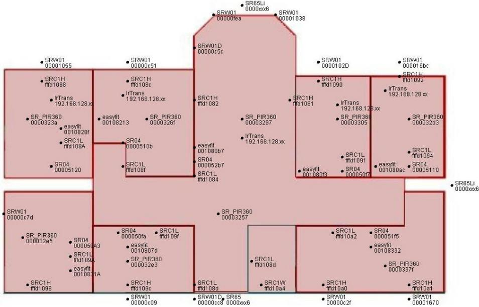
Figure 2.4: Plan over all the sensors installed in the building.
