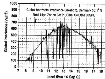
Figure 4: Global radiation data collected using a 80spc and a Kipp-Zonen CM21 around the spring equinox in Denmark.
