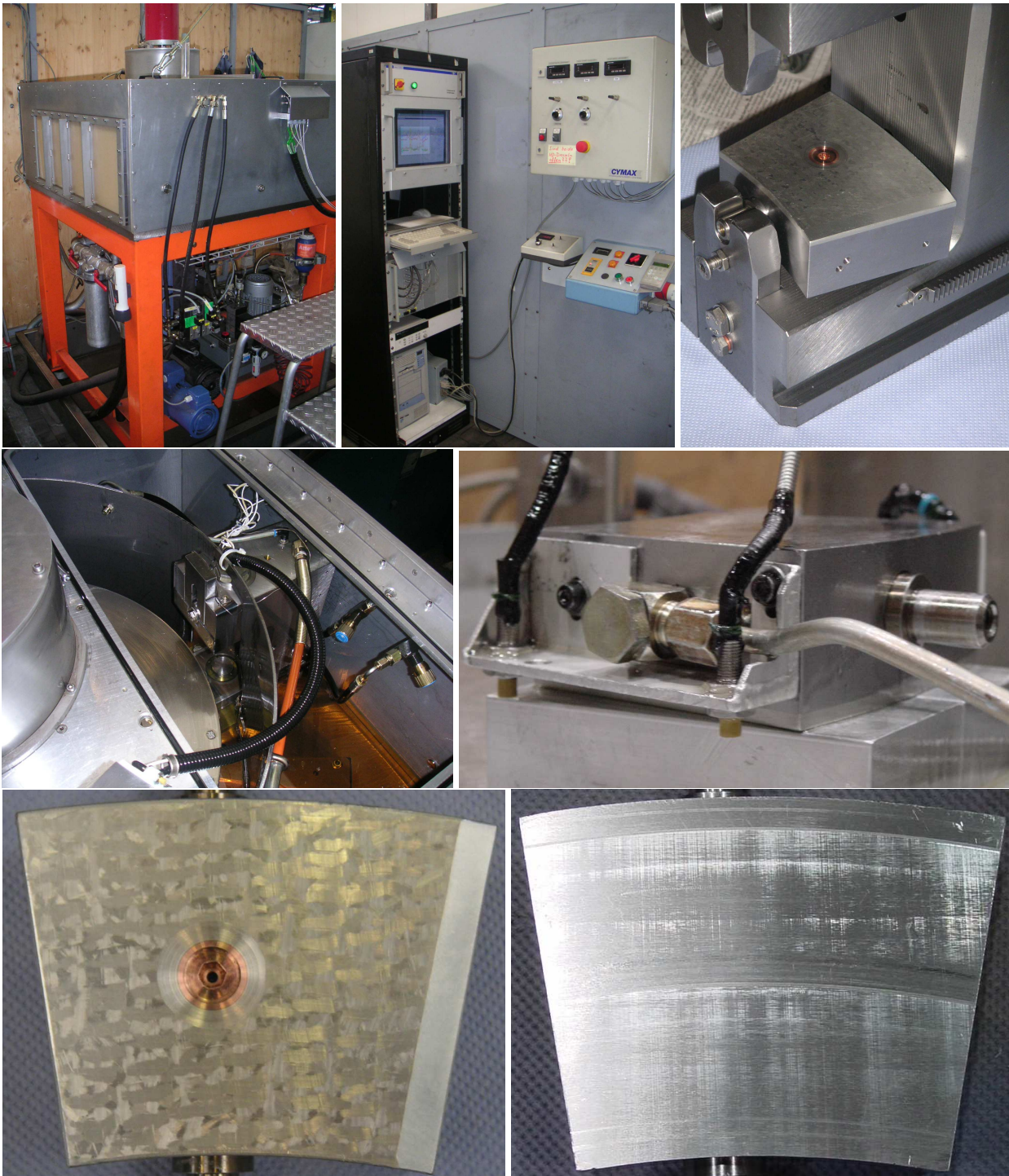
Figure 4.3: Top left: The test-rig. Top middle: The user interface. Top right: Pad shown in a dismantled pad holder. Middle left: A view into the test-rig with a dismantled pad. Middle right: A view of the trailing edge. The distance sensors and the oil injection pipe is seen. Bottom: Pictures of the tested pads taken after the measurements. The plain pad has a ground down surface finish.
