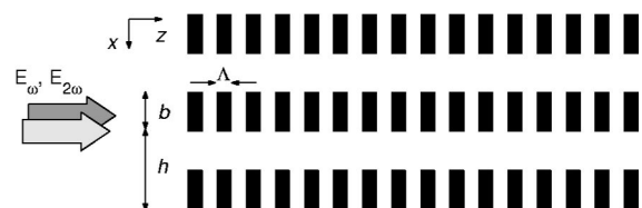
FIG. 1. Schematic top view of grating design of QPM structure.
