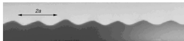
FIG. 1. Side view of a vortex ripple pattern under oscillatory flow in a long, slender channel (courtesy of J.L. Hansen). The arrow indicates the amplitude of the fluid oscillations in the bulk.
