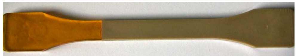
Fig. 3 Injection moulded 2K test specimen (PEI-first shot and PEEK-second shot)
