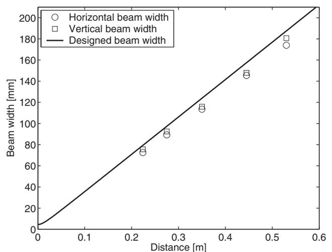
FIG. 6. Gaussian widths of the beam leaving the horn antenna. The horizontal and vertical beam widths should be identical, as the horn has a circular symmetry. The error is less than 3% between the measured beams in two orthogonal directions. The solid line represents the designed beam width.
