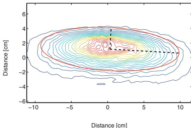
FIG. 8. (Color) Contour plot shows the radiation intensity in the  $y$ - $z$ -plane at a distance of 166 mm from the reference point (see Fig. 7). The dashed lines show the width in the direction of the major axes of the anisotropic beam.
