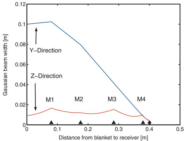
FIG. 3. (Color) Gaussian beam widths in the two orthogonal directions in the transmission lines. Between the reference point and mirror M1, the two orthogonal directions coincide with the *y*-axis (blue curve) and the *z*-axis (red curve). The triangles indicate the mirror positions M1 to M4 and the diamond indicates the position of the waist which is located slightly inside the horn antenna. See also Fig. 7.
