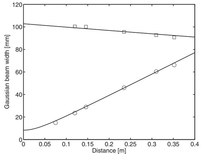
FIG. 9. Propagation of the  $y$ - and  $z$ -component of the anisotropic Gaussian beam into the vessel. The squares show the horizontal component and the circles show the vertical component. The solid lines represent the calculated beam widths. See also Fig. 7.
