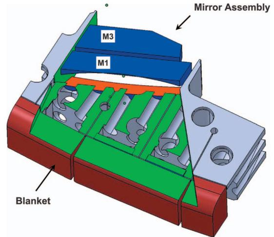
FIG. 5. (Color) Mirror assembly for the proposed antenna on the HFS integrated in the blanket of the inner wall of ITER. The cutting surface of the blanket is depicted in green. Only the mirrors M1 and M3 (blue) and the surface of mirror M2 (red) of the mirror assembly can be seen. See also Figs. 4 and 7.
