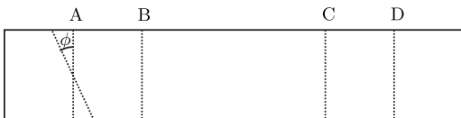
FIG. 11. Top-view schematic of chip and blades (A)–(D). In the FEM analysis, each blade is rotated an angle \phi . The stress distribution for different configurations of blade rotation is listed in Table II.
