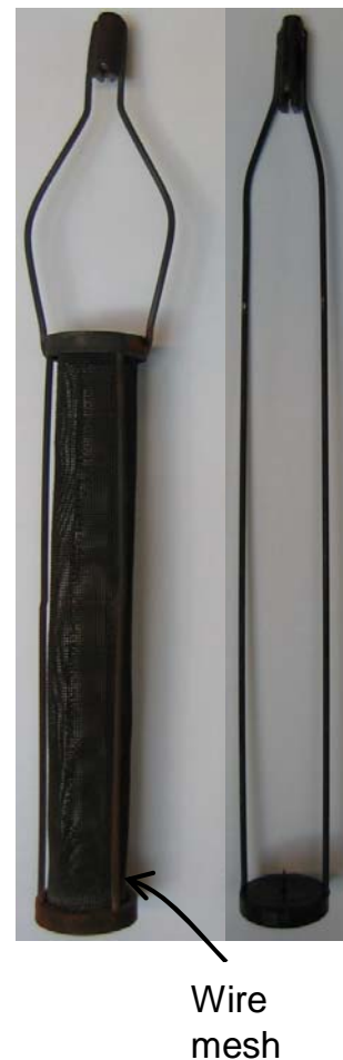
Figure 4-11: Sample holders used for devolatilization investigation of large particles in the Macro TGA setup ( \text{\O} = 18 shown). Not to scale.
