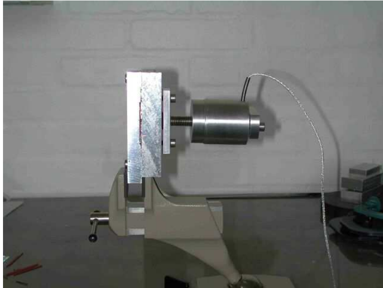
Figure 7.7: The photo shows our bonding force set-up clamped into a vice. The clamped part held the microsystem being tested, while the cylindrical part next to it on the right could be screwed into the holder. To the utmost right was a load cell (ELA-B1E-500N, Entran, Ludwigshafen, Germany), that exerted a certain force on the test system. It was possible to record the forces on-line as shown in Fig. (7.9). The technical drawing in Fig. (7.8) explains the details of this photo.
