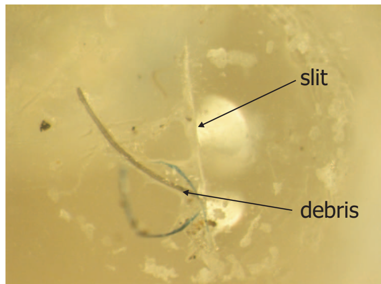
Figure 2.21: Debris caught inside the incision prevented complete closing of the membrane and led to failure of the valve.
