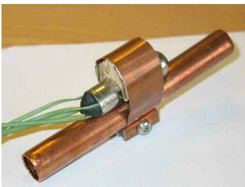
Figure 7-11: Wooden brick as insulation between strap and bulb
