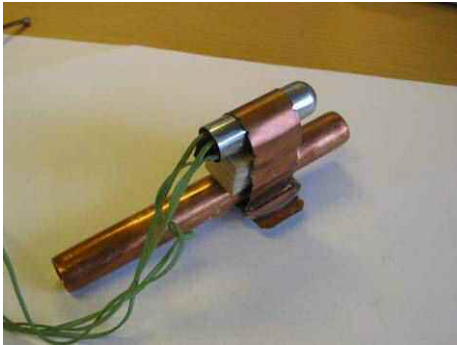
Figure 7-13: Wooden brick as insulation between pipe and bulb
