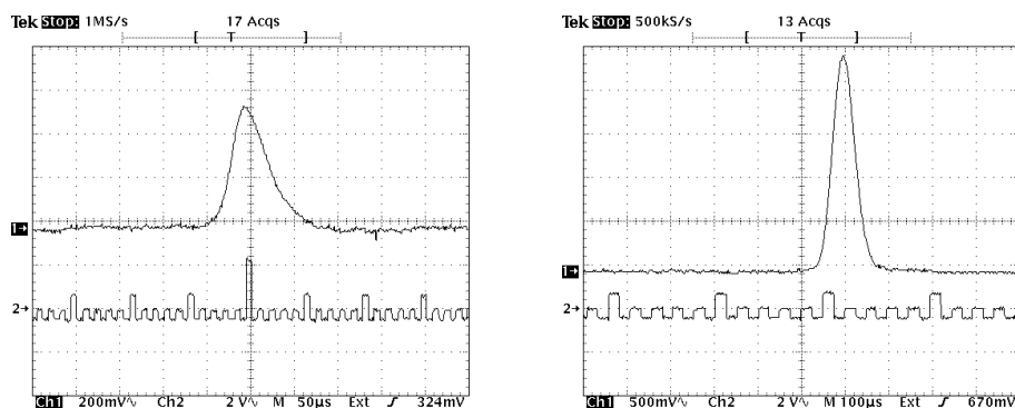
Figure 2.6: Line widths of the simple Ti:Sapphire laser using different BRF elements. Single plate filter to the left, three plate filter to the right.
