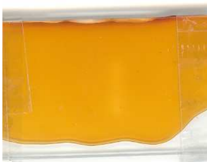
Figure E.2: Bleaching of gellified sample. The bleached area is visible on the centre-right of the image. The 400 nm beam for bleaching was approximately 1 mm in diameter, and the scanned length was 9 mm. On the sample the bleached area is approximately 2 mm wide and 10 mm long, the widening of the area is due to diffusion of the chromophores. The scanning was done in the afternoon, and next morning the diffusion had completely wiped out the bleached area.
