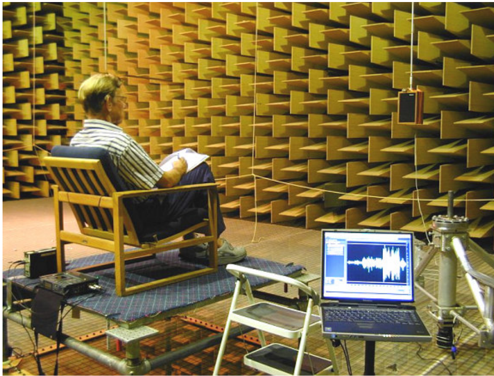
Figure 4.13. Test subject listening to compressed signals in the anechoic chamber. All subjects wore bin-aural BTE hearing aids, fitted linearly to NAL-R for the individual hearing loss – amplifying the compressed signals presented from the loudspeaker.
