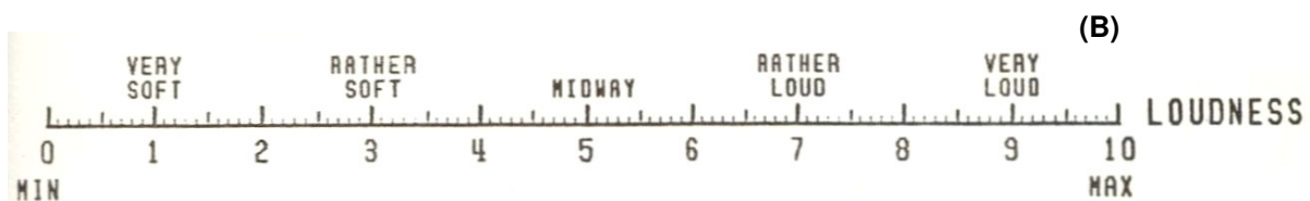
Figure 2.9. Two examples of categorical loudness scales. In (A) the touch-screen with 11 categories used by Launer (1995). In (B) the interval-scale with five main categories used by Gabriellson et al (1985). In that scale, subjects mark the perceived loudness with a pencil or pen.
