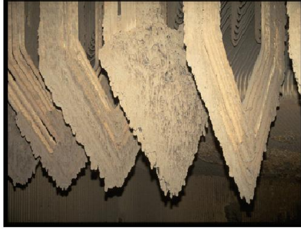
Figure 2.5: An example of deposit formed on the superheater during pulverized biomass combustion
