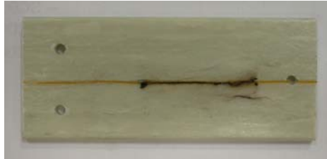
Figure 5.7 Specimen P9, where the tracking erosion occurred along a fibre bundle with different characteristics in the surface.
