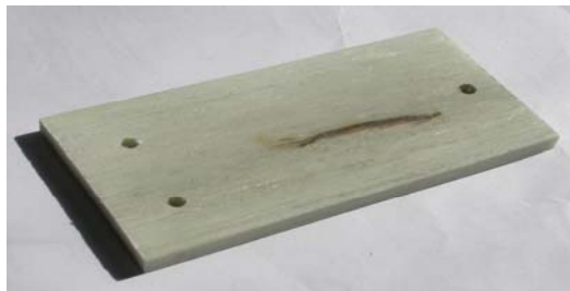
Figure 5.6 Specimen P12, where fibres located in the uppermost surface layer are the main cause of the fast deterioration.
