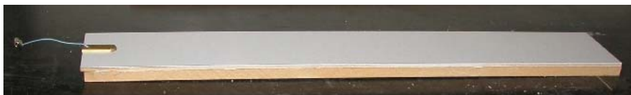
Figure 5.55 Test specimen with brass electrode mounted on the surface as simulated receptor.
