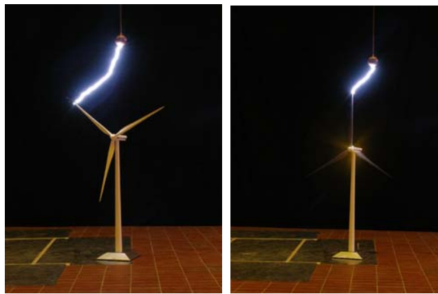
Figure A24 Discharges to a scale model of a Vestas V90 wind turbine
