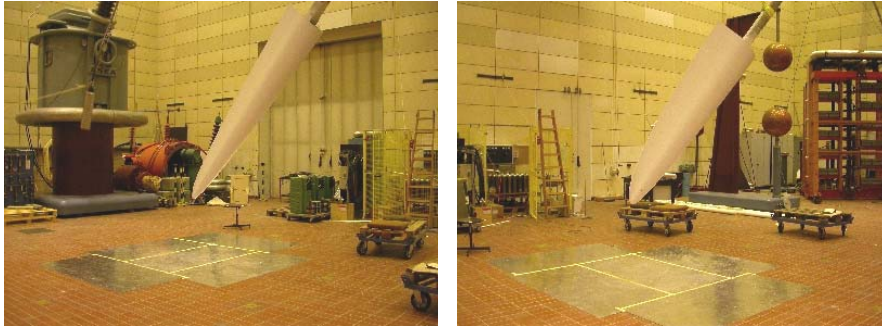
Figure 6.5 A 3m GFRP blade tip fixed by its 3m beam elevated above the ground electrode in position A8.
