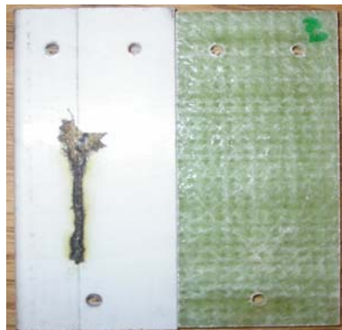
Figure 5.8 Characteristic erosion of specimens with different resin systems. Left: Specimen P13 with a polyester based resin, Right: Specimen E20 with an epoxy based resin.
