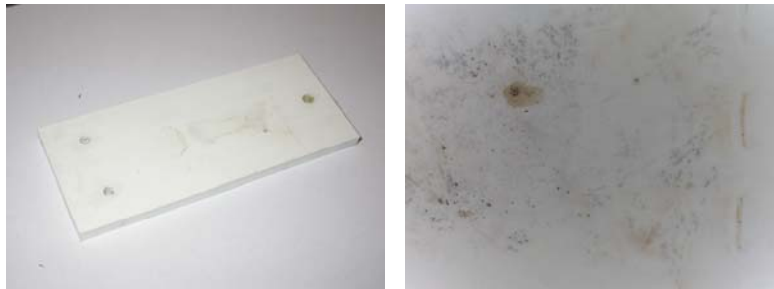
Figure 5.4 Specimen P7 with a uniform and widely distributed impact exhibiting tiny pin-holes.
