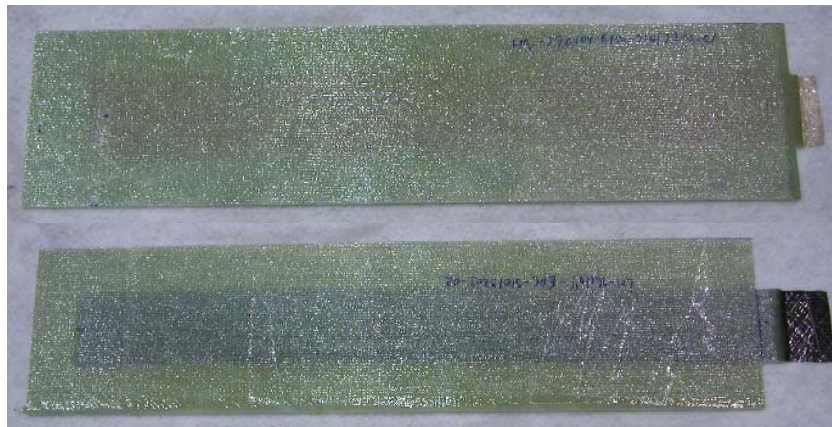
Figure 5.27 Specimens with flat ground electrodes. Top: Copper mesh electrode, Bottom: CFC electrode.
