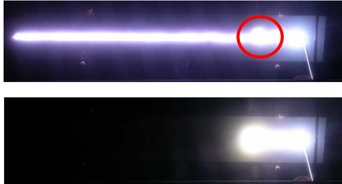
Figure 5.25 Image of breakdown in specimen (L). Note the strong light on the first picture indicating a pre-breakdown.
