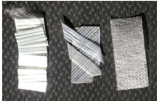
Figure 5.9 Different ways of organising glass fibres, as uniformly oriented fibre bundles, perpendicular woven mats with an angle between laying direction of 90 deg and as a felt structure ensuring randomly oriented fibres.
