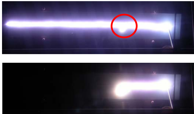
Figure 5.26 Image of breakdown in specimen (M). Note the strong light on the first picture indicating an initial breakdown.
