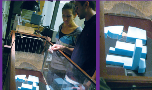
Study of the ground-near wind conditions on Axeltorv in Copenhagen performed in the wind tunnel at DTU Civil Engineering. Miriam Ann Hellmann and Victor August Aalund-Olsen, students in Architectural Engineering, conducted their BSc project within the framework of a research collaboration between DTU Civil Engineering and Gehl Architects. Photo: Holger H. Koss
