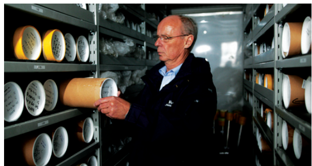
The soil samples taken from 50-100 m below the seabed are stored in container under controlled climatic conditions. Photo: Femern A/S
