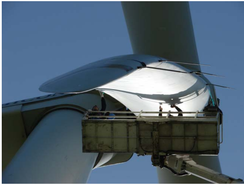
Figure 8 The local inflow at four radial positions was measured with four five hole pitot tubes sticking out from the leading edge of the blade.
