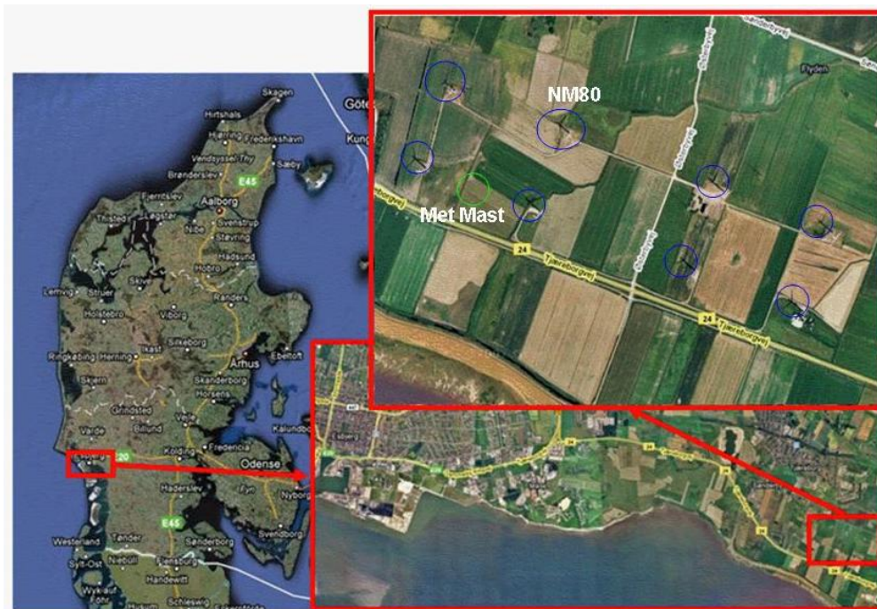
Figure 9 Map of the site (maps.google.dk). The site is app. 10 km east-south-east of Esbjerg. The site has eight wind turbines of the size around 2MW. The position of the NM80 is shown together with the other 7 turbines on the site. Also the position of the meteorology mast is shown.
