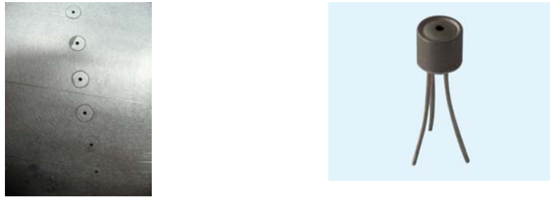
Figure 1 Microphones with a diameter of around 4 mm installed about 1 mm below the blade section surface and connected through a boring of 1.5 mm.
