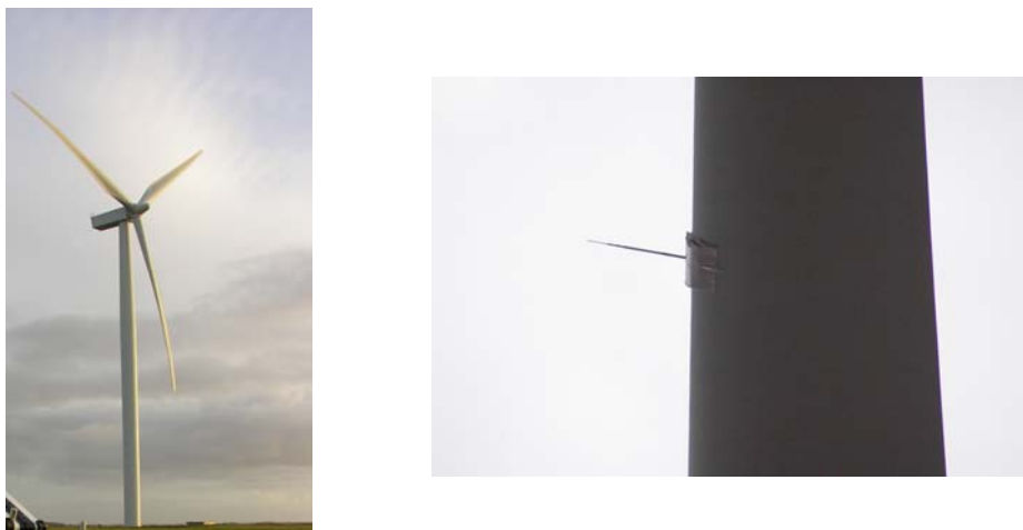
Figure 3 The five hole pitot tube mounted in radius 36 m on the blade in a distance of about 0.80 m in front of the leading edge of the blade. Rotor diameter is 107 m.
