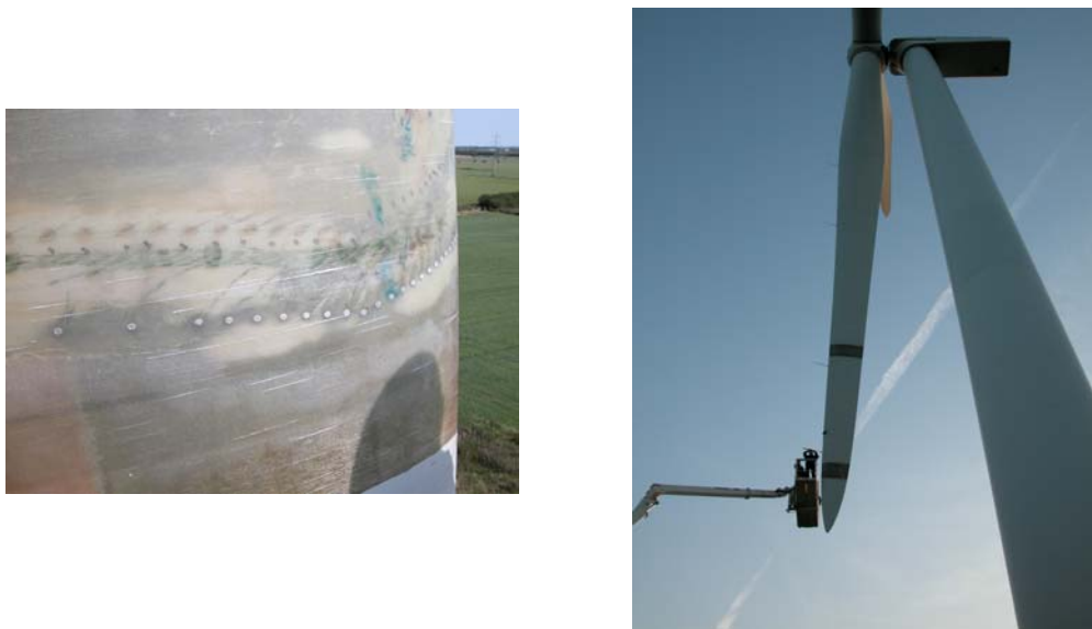
Figure 7 To the left: about 50 microphones were installed about one mm below the blade surface at the outboard section at radius 37 m for high frequency surface pressure measurements. The boring from the microphones to the blade surface has a diameter of 1.5 mm. To the right: every evening all pressure taps, microphones and five hole pitot tubes were covered with tape to protect against moisture and rain.
