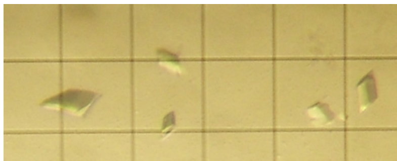
Figure 9.3 Crystals of cgTPH1 grown in 0.2 M MIB buffer pH 8.5, 22.5% PEG 10000, cgTPH1 concentration 3.5 mg/mL. One square in the mesh is 90 \times 90 \mu\text{m} .
