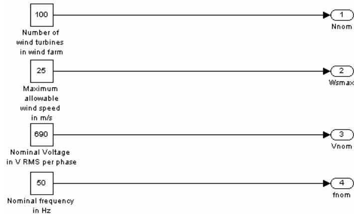
Fig. 35. Layout of the subsystem »Wind farm basic properties«; this subsystem consist of a set of constants, which are set, and is as such a passive subsystem. (The data values are sample data).
