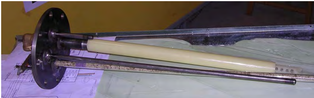
Fig. 3-3 Prototype example showing a thin PEX pipe (with holes at the end) with an additional thick PEX pipe to decrease the heat transfer coefficient.
