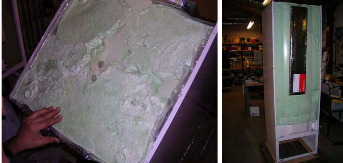
Fig. 3-2 Left: View of the top of the tank with vacuum panels at the sides and the 2 small holes for the temperature sensors in the middle of the tank; Right: View of front of the tank without the cover plate to see one of the vacuum panels.
