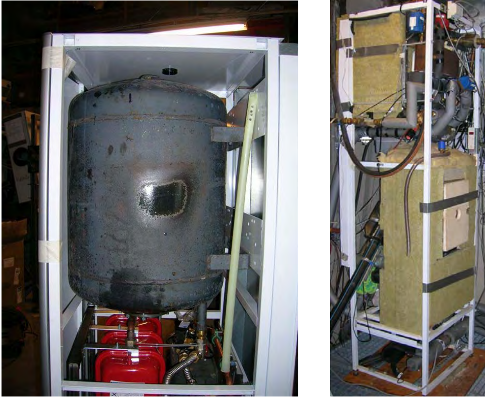
Fig. 3–9 Left: Top of the technical unit with a standard 80 liter auxiliary tank instead of a gas boiler. Right: Prototype of a technical unit at SERC with a cubic 80 liter tank in the top and an adapted pellet stove below.
