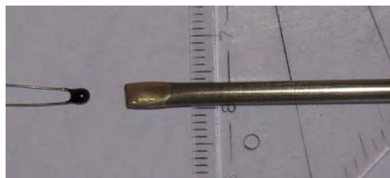
Fig. 5–6 A thin and long stainless steel needle (right) is used as a sensor pocket for a very tiny NTC sensor element (left).
