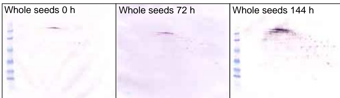
Figure 3.32. Detection of LD in 2D western blots of whole seed barley protein extracts using LD antibodies. 20 \mu L loaded on each gel (~20-50 \mu g protein)
