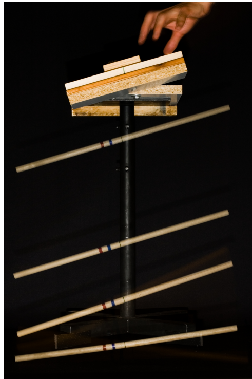
Figure 4.2: Fixture used to help drop dowels in a uniform manner on every trial. Dowel being dropped in photo is 45 cm long.
