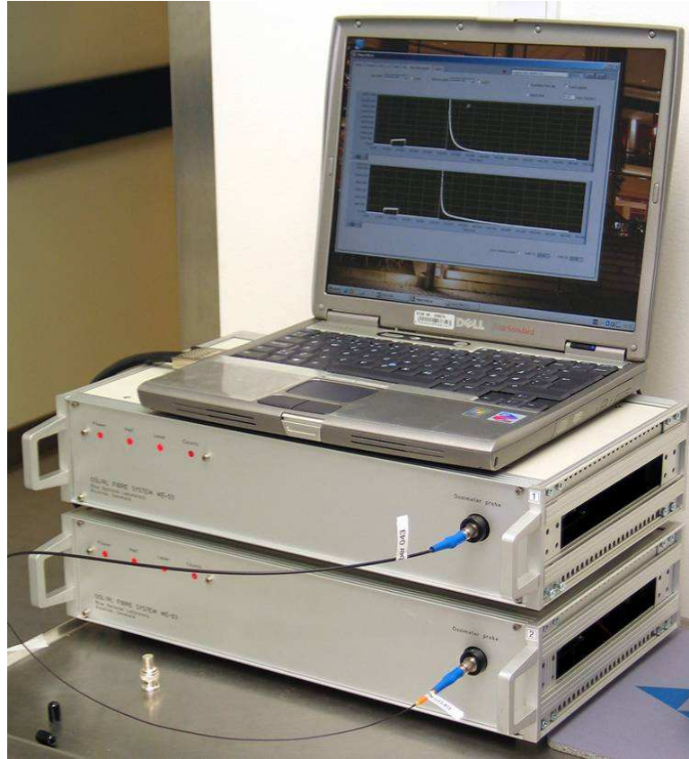
Figure 3.1: The fiber system ME03. Two readers are stacked on top of each other each having one fiber cable attached. A laptop controls both readers and the RL and OSL signals from the two probes can be seen in the Labview program interface.
