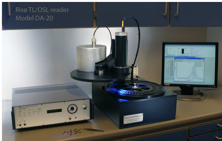
Figure 3.3: The latest version of the Risø reader (TL/OSL-DA-20). To the left is shown the minisys system which provides the basic low-level commands to the reader (middle). The experimental sequences and data collection can be handled from a windows based software (right).
