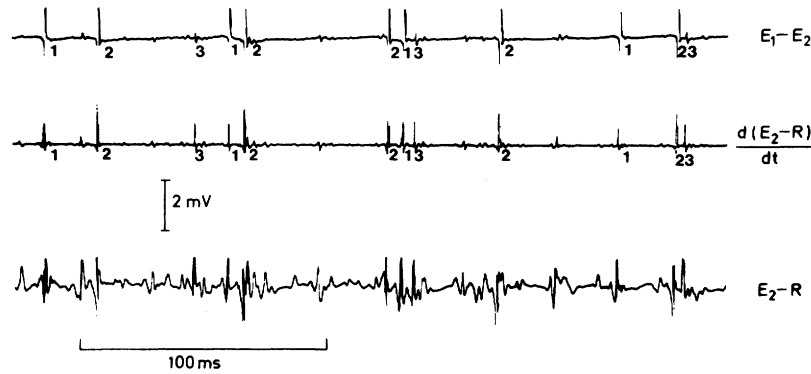
Fig. 11. Above: Selective recording of action potentials from two motor units 1 and 2 via a side hole electrode in the anterior tibial muscle of a normal subject at 20% of maximal effort. Middle: Action potentials from three motor units (1, 2, and 3) selected by differentiation of the lower trace: d(E_2 - R)/dt . Note the similar shape of the potentials from motor units 1 and 3. Below: Summated activity from many motor units recorded between one of the recording surfaces of the side hole electrode and a reference electrode ( E_2 - R ).
