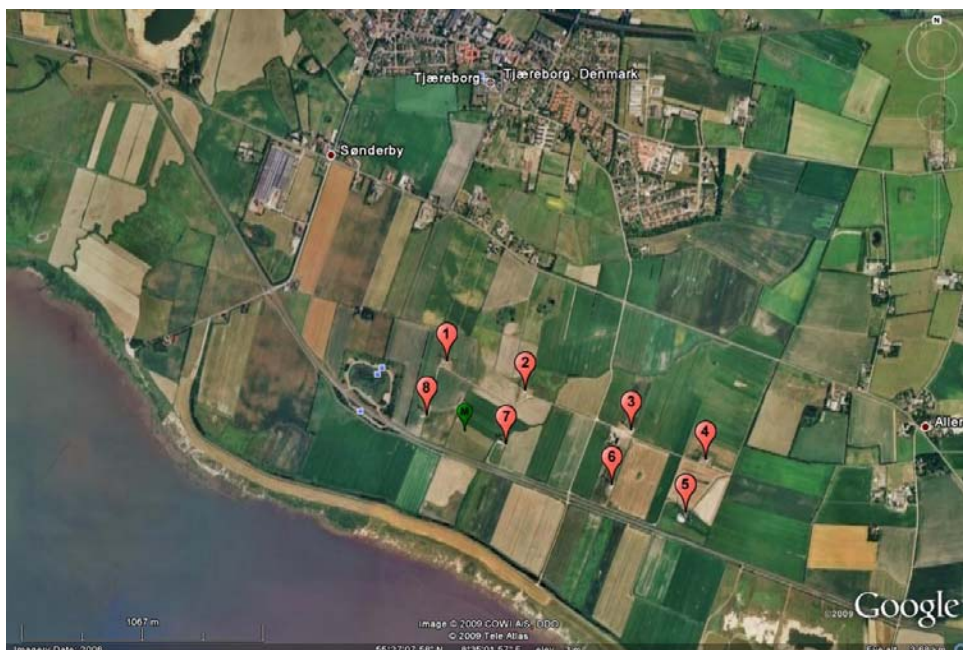
Figure 1.3 The landscape of the area of the experiment where 8 wind turbines are located (Google Earth ® ). The lidar was mounted in the NM80 turbine indicated by #2 and the MET mast providing data for the experiment is indicated by M.
