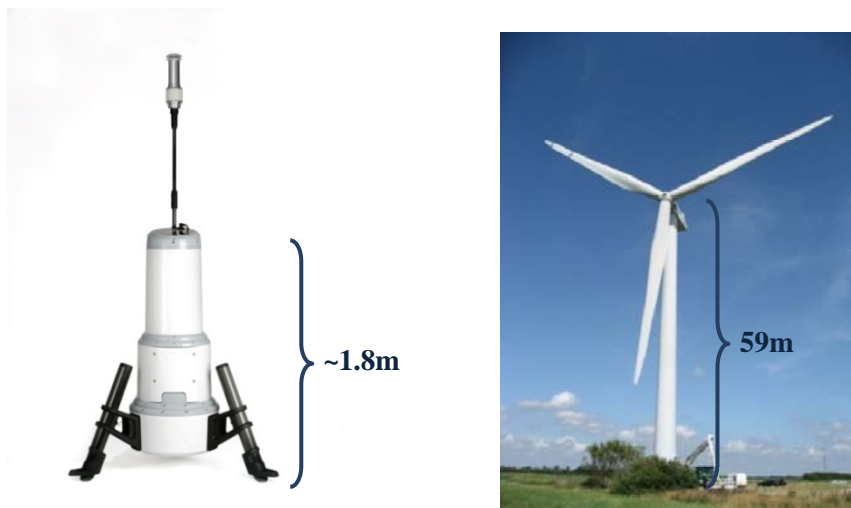
Figure 1.1 Photos of the QinetiQ (Natural Power) ZephIR lidar system (left) and the NM80 (Vestas) wind turbine (right).
