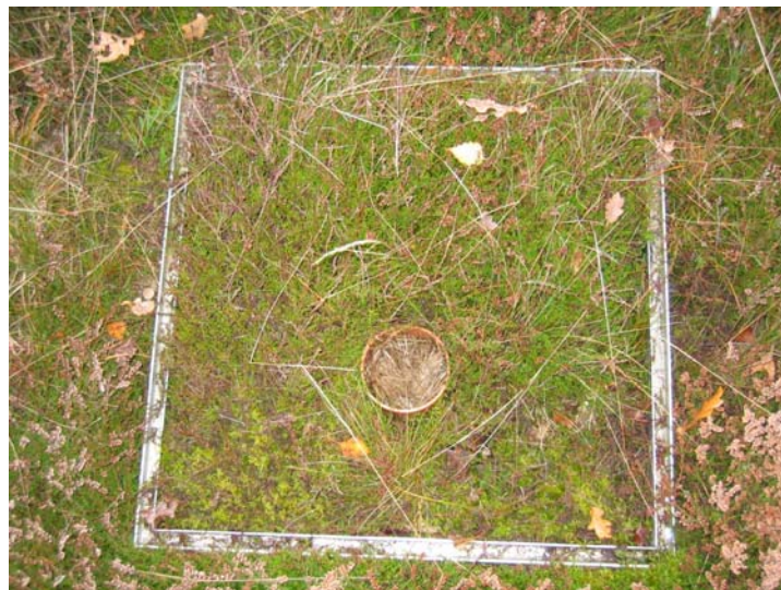
Figure 8. Bases for flux measurements. The large frame for ecosystem fluxes, small collar without aboveground vegetation for soil respiration fluxes.
