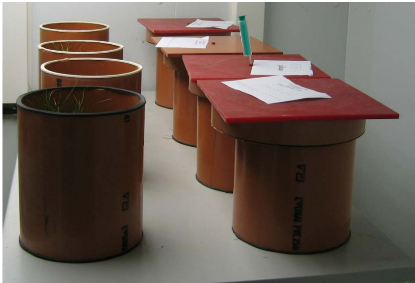
Figure 2. Respiration measurements of mesocosms, open chambers to the right, closed chambers at left.
