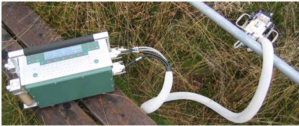
Figure 9. Soil respiration was recorded by the Li-Cor 6400.
