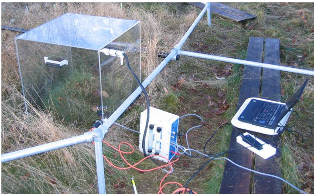
Figure 10. The ecosystem flux chamber connected to a CIRAS DC 10 measuring net ecosystem exchange of CO_2 .
