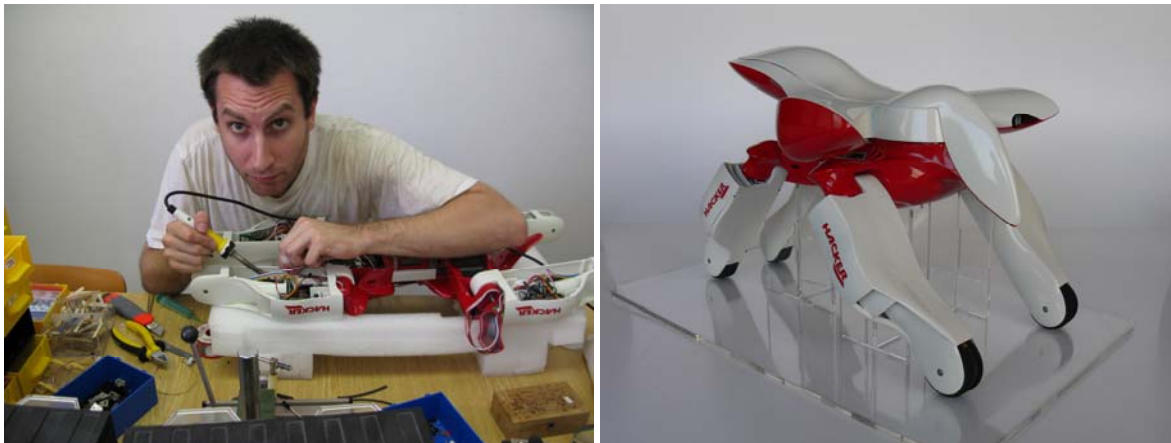
Figure 3 Student working on RobotX – project of mobile robot with hybrid undercarriage.
