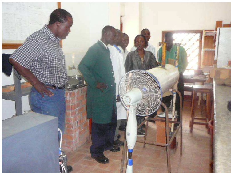
Figure 1: locally-constructed tunnel dryer
