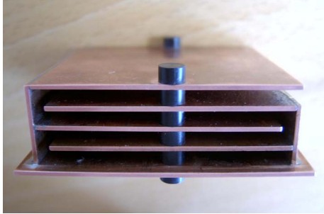
Fig. 4. The fabricated 4-layer patch antenna with a small ground plane, in design 7, operated at 415 MHz
