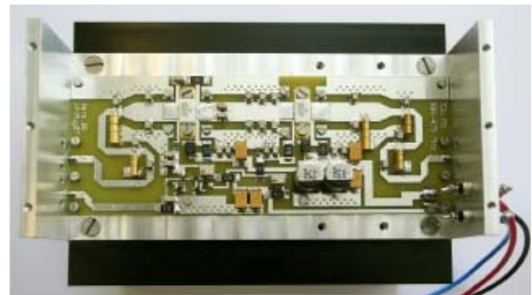
Fig. 3. Purpose-build Power Amplifier module.
