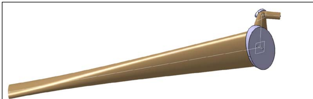
Figure 25: Mirrors and beam shape for the CTS LFS launcher beam
