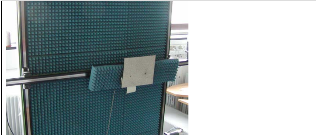
Figure 5: Detector diode mounted on a translation stage and moving in two dimensions.
