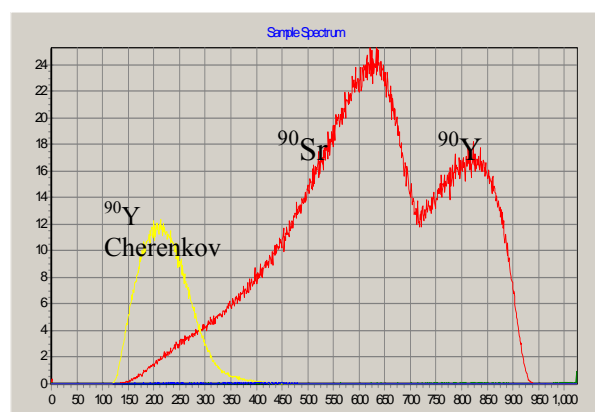
Fig.5 Cherenkov spectrum of Y-90 and beta spectrum of ^{90}\text{Sr}/^{90}\text{Y}
