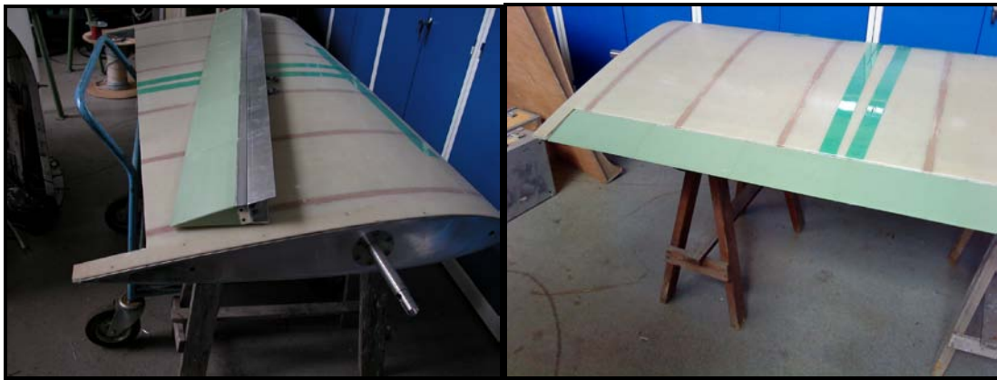
Figure 6 On a 1.9 m long NACA0015 airfoil section model with a chord length of 1 m, six of the flap prototypes were glued together and then attached to the airfoil section model.
