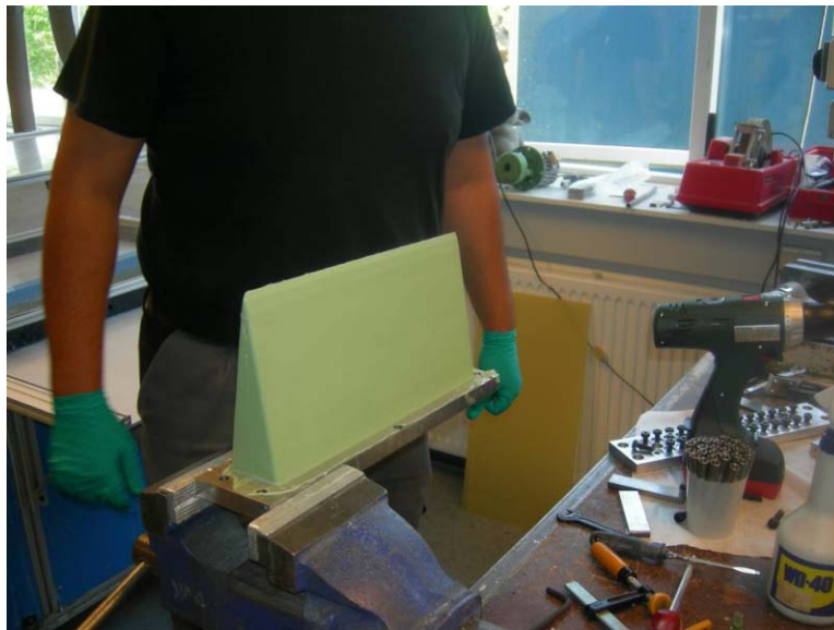
Figure 3 Manufacturing of prototypes was carried out by the Material Research Division at Risø DTU. Different silicone rubber types were tested.
