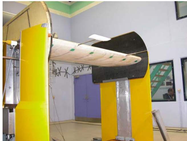
Figure 10 Two different inflow sensors were tested: a five hole pitot tube and a small sensor airfoil mounted on a rod with a strain gauge giving a signal proportional to the lift on the sensor airfoil.
