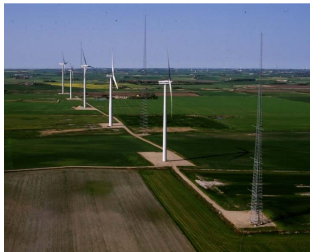
Figure 2-2 The row of wind turbines at the Høvsøre test site with the tall met. mast in the front.
