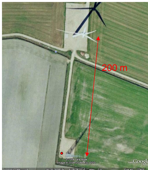
Figure 2-5 Distance between met. mast and wind turbine at test stand 5 (picture from Google Earth). The location of the tested lidars is indicated by the red dot.
