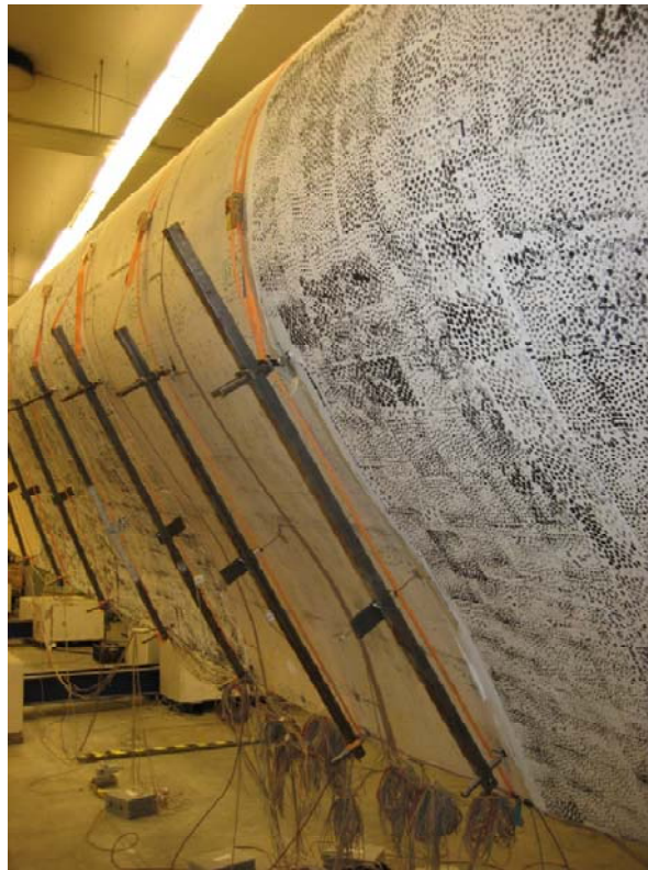
Figure 2. LT-NTs mounted on the blade
