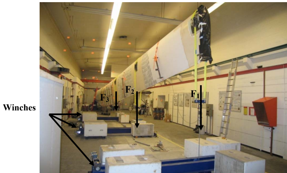
Figure 2.2. The blade with the measurement equipment mounted on the test rig.
