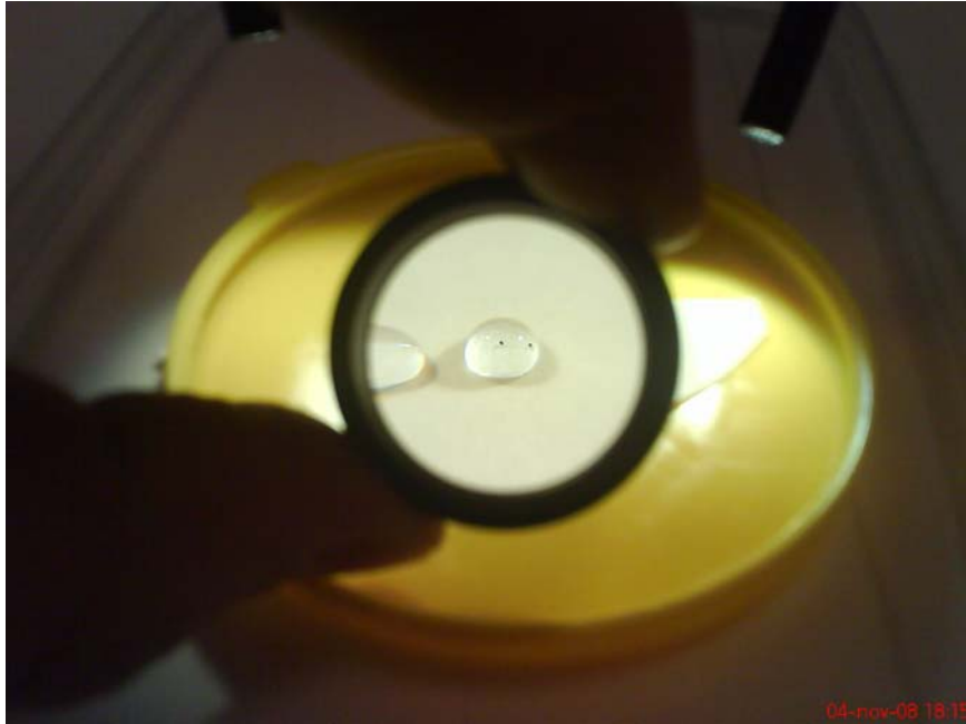
Figure 4. Two isolated Thule actinide particles placed in a drop of water. Photographed using an ordinary loupe and a camera with macro settings. The particles were about 50 \mu\text{m} and had an activity of 55 and 40 Bq ^{241}\text{Am} respectively.
