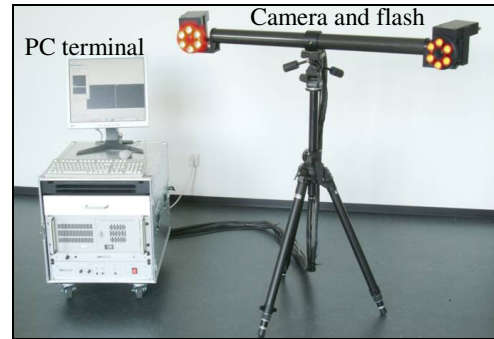
Figure 2 : Stereo Camera system PONTOS, with tripod, cameras and flashes
