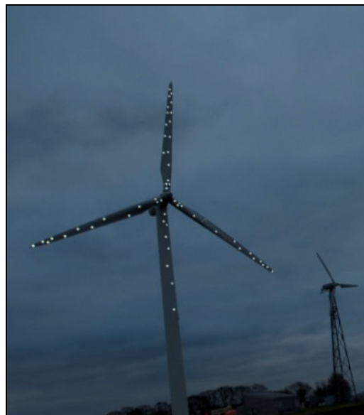
Figure 5 The effect of flash on the reflective markers. Wind turbine at campus, Dec 2007.
